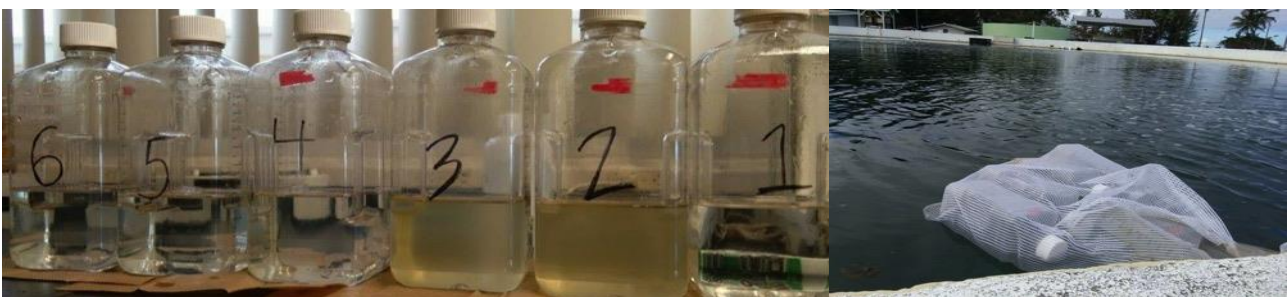
Fig. 2: Left: Culturing bottles on day 3 of sampling. Notice bottle number 1, which stopped growing after day 2 and was taken out of the growth calculations, Right: bottles floating in a pond at PACRC to allow sunlight and regulate water temperatures.
