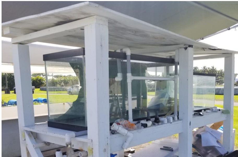
Figure 2. Wooden stand with 75-gallon and 20-gallon glass aquariums with plumbing leading to 50-gallon plastic sump (not pictured).
